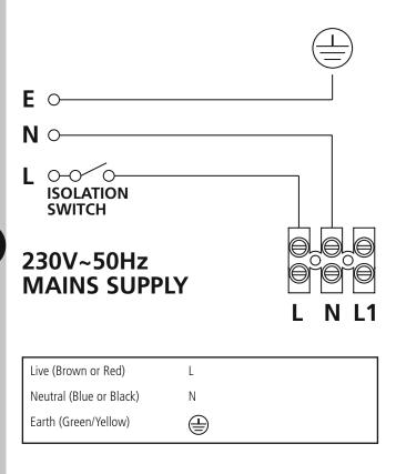
• The diagram below also shows the required connections for the addition of slave luminaires. When adding slaves, be sure not to exceed the Total Switchable Loads (see section 3. Technical Specifications).
